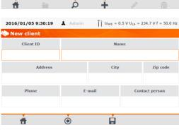
Press each field and enter client's data with on-screen keyboard. Filling data marked with orange frame is mandatory.
