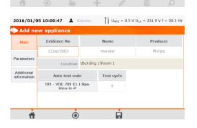
Enter (type) appliance's data in the same way as for the client or object. Filling data marked with orange frame is mandatory. Additional data is available under **Parameters** and **Additional information**.
