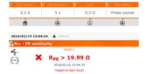
Negative test result: R<sub>PE</sub> > LIMIT
