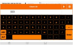
Press to toggle between next and previous data field without disabling the keyboard. After entering all data confirm
