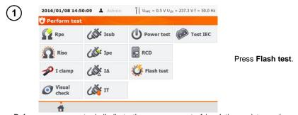
Before measurement, similarily to the measurement of insulation resistance (see sec. 4.3), following parameters must be set: **test voltage** (1500 V lub 3000 V), **test duration** and **limit**.
