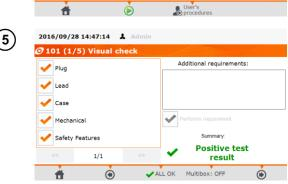
For this example: after initial visual check, select proper fields on the left side of the screen (confirming or not the correctness of the statement). Press
