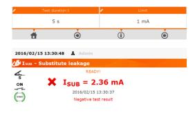
Negative test result: I<sub>SUB</sub> > LIMIT
