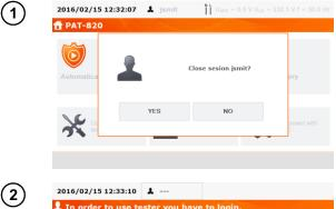
To change user, the current one has to log out. Press his name on the top of the screen in the main menu and then pressYES to confirm.
