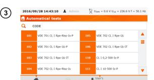
Select the test number from the list or scan the code from the proper barcode (or 2D code) with the barcode reader (PAT automatically detects connected barcode reader). If the test method was previously assigned to the selected appliance, it will now be highlited.
