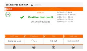
Appliances with RCD - AUTO mode tests, see section 4.13.
