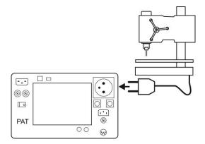
For Class II and accessible parts disconnected from PE in Class I, connect the probe to **T2** terminal socket and touch the accessible parts of the tested device.
