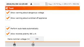
If each test is meant to be executed one after another automatically Perform auto-tests automatically option must be selected. Otherwise each test will be executed separately by pressing START button.
