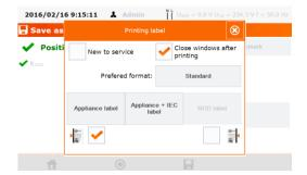
Managing the printer is on: Select the appliance in the database (or add a new one) and after selecting of the choice, press , the appliance will be selected. Select proper checkbox if the device is being tested for the first time, and another checkbox for chosing how to mark label with the side stripe (for retest period). Click the button with selected type of label - the label is printed and the result is recorded. Closing the window using button
