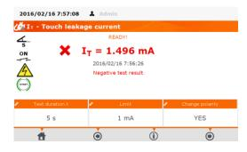
Negative test result: I<sub>T</sub> > LIMIT
