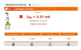
Negative test result: I<sub>PE</sub> > LIMIT
