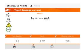
3 Connect the mains plug of the tested device into the test socket of the tester. Use the probe connected to T2 terminal socket and touch the accessible parts of the tested device. (For Class I devices - touch acessible parts disconnected from PE).
