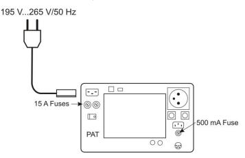
Two 15A fuses protect L and N lines from the supply socket to the test socket, they are tripped when current consumption from the test socket is too high (>16A).
